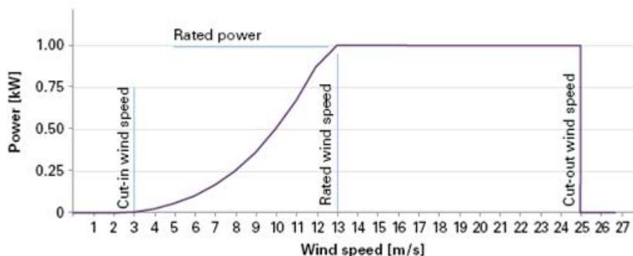
The ratio of Actual Output to the theoretical maximum Rated Output is known as the Load Factor. i.e. Actual Output = Load Factor x Turbine Rating x 8760 hours/year
