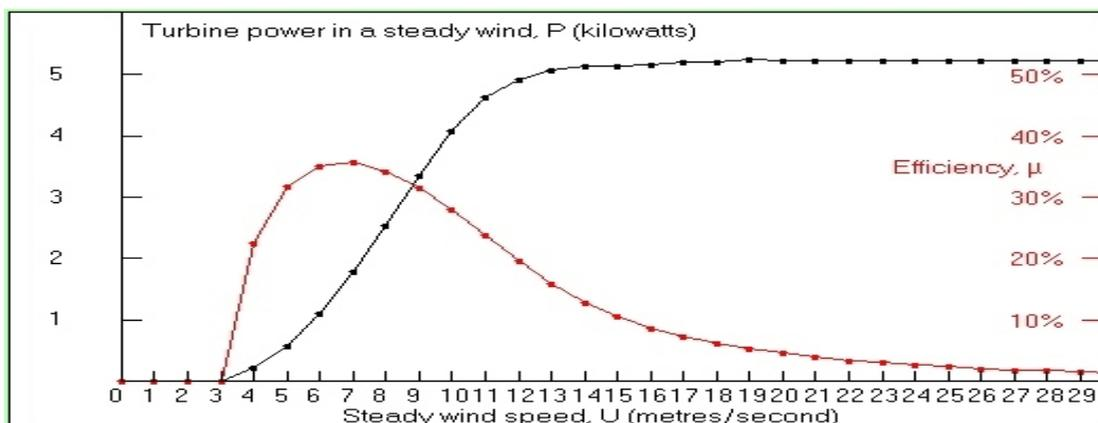
The ratio of Actual Output to the theoretical maximum Rated Output is known as the Load Factor i.e. Actual Output = Load Factor x Turbine Rating x 8760 hours/year
